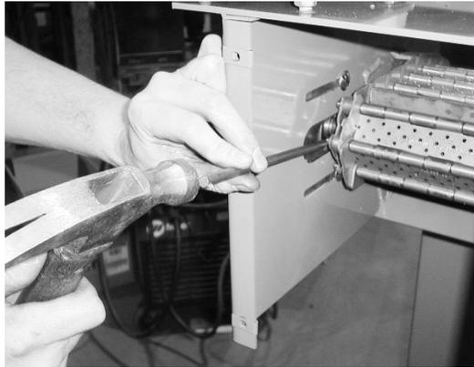
**Figure 15: Removing the Axle Pin**
