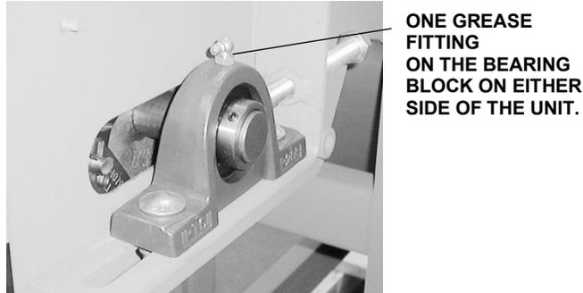
**Figure 30: Grease Fitting Location**
